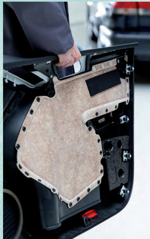
Fibres for lightweight automotive composites such as door panels.
